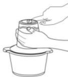
Note: Please hold the plastic part of the blade handle when assembling or disassembling the blade, and do not touch the blade to avoid injury.
